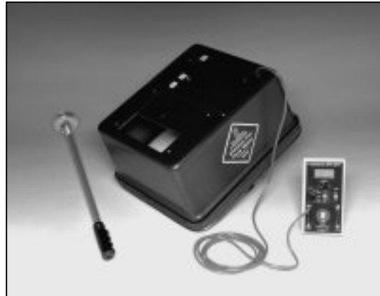
Exhaust Fan Flow Meter with DG-3 Pressure Gauge
